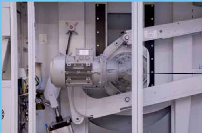
Combined drive motor and planetary gear.
