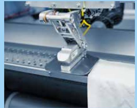
6 When releasing the corner of the linen to the vacuum beam, the clamps move sideways, and straighten out the corners of the linen.
