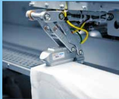
5 Fast, yet gently spreading of the linen onto the vacuum beam
