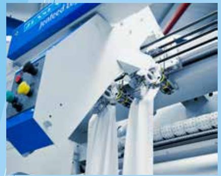
3 Transfer from the EasyClamps to the Soft-Touch spreading clamps
