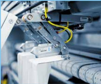
4 The Soft-Touch spreading clamps pivot to a horizontal position and start spreading the linen
