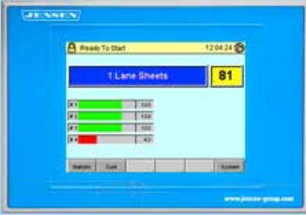
Jentrol HMI PLC and control system with touch screen.
