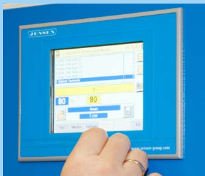
Jentrol HMI PLC and control system with touch-screen
